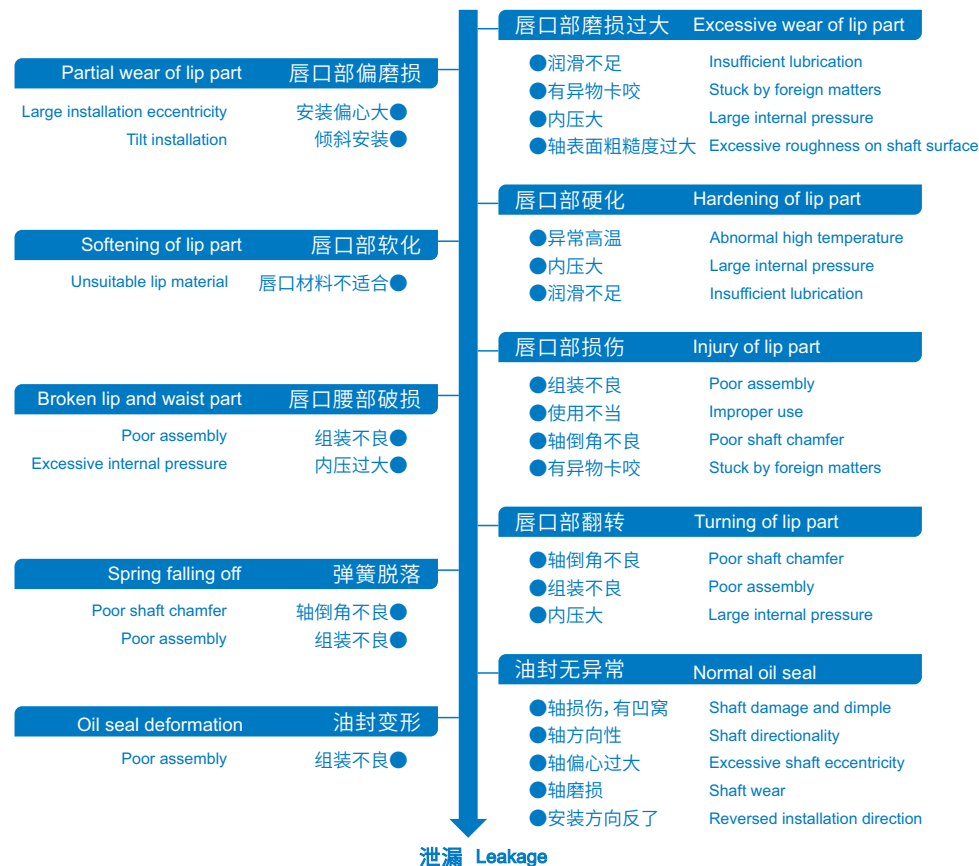
Figure 5-1 由唇口部泄漏的主要原因 Schematic diagram of main causes of leakage from lip part
